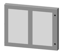
Saginaw universal deep-hinged door, NEMA 3R/4/4X/12/13,  $22.00 \times 28.00 \times 2.63$ in, 304 stainless steel, concealed hinges, polycarbonate window. For use with wall-mount enclosures.
