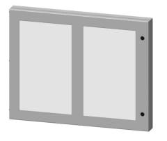
Saginaw universal deep-hinged door, NEMA 3R/12/13, 22.00 x 28.00 x 2.63in, carbon steel, RAL 7035 light gray, concealed hinges, polycarbonate window. For use with wall-mount enclosures.
