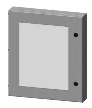
Saginaw universal deep-hinged door, NEMA 3R/12/13,  $22.00 \times 18.00 \times 2.63$ in, carbon steel, ANSI 61 gray, concealed hinges, polycarbonate window. For use with wall-mount enclosures.
