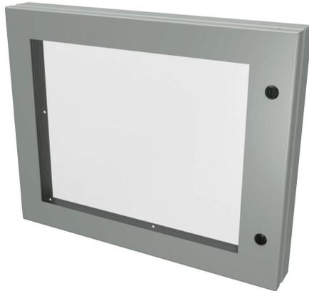
Saginaw universal deep-hinged door, NEMA 3R/4/12/13, 16.00 x 20.00 x 2.63in, carbon steel, ANSI 61 gray, concealed hinges, polycarbonate window. For use with wall-mount enclosures.
