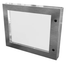
Saginaw universal deep-hinged door, NEMA 3R/4/4X/12/13, 16.00 x 20.00 x 2.63in, 304 stainless steel, concealed hinges, polycarbonate window. For use with wall-mount enclosures.
