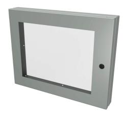
Saginaw universal deep-hinged door, NEMA 3R/4/12/13,  $14.00 \times 18.00 \times 2.63$ in, carbon steel, ANSI 61 gray, concealed hinges, polycarbonate window. For use with wall-mount enclosures.
