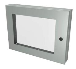
Saginaw universal deep-hinged door, NEMA 3R/4/12/13,  $12.00 \times 16.00 \times 2.63$ in, carbon steel, ANSI 61 gray, concealed hinges, polycarbonate window. For use with wall-mount enclosures.
