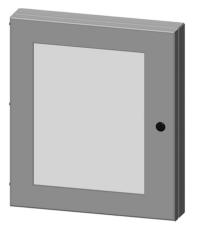
Saginaw universal deep-hinged door, NEMA 3R/4/12/13, 12.00 x 12.00 x 2.63in, carbon steel, ANSI 61 gray, concealed hinges, polycarbonate window. For use with wall-mount enclosures.
