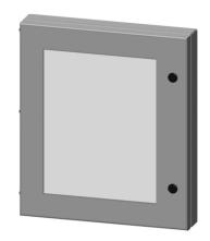
Saginaw universal deep-hinged door, NEMA 3R/4/4X/12/13,  $12.00 \times 12.00 \times 2.63$ in, 304 stainless steel, concealed hinges, polycarbonate window. For use with wall-mount enclosures.
