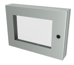
Saginaw universal deep-hinged door, NEMA 3R/4/12/13,  $10.00 \times 14.00 \times 2.63$ in, carbon steel, ANSI 61 gray, concealed hinges, polycarbonate window. For use with wall-mount enclosures.
