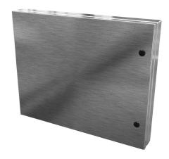
Saginaw universal deep-hinged door, NEMA 3R/4/4X/12/13,  $16.00 \times 20.00 \times 2.63$ in, 304 stainless steel, concealed hinges. For use with wall-mount enclosures.
