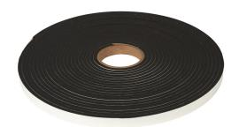
Saginaw strip gasket, replacement, self-adhesive, closed-cell urethane, 1/4in thick x 3/4in wide x 50ft long roll. For use with NEMA 4/4X enclosures.
