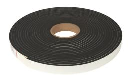
Saginaw strip gasket, replacement, self-adhesive, closed-cell urethane, 1/4in thick x 1in wide x 40ft long roll. For use with NEMA 4/4X enclosures.
