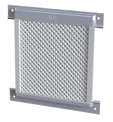
Saginaw filter, replacement, 14.14 x 8.25in, aluminum mesh, aluminum frame, washable. For use with SCE-AVK812 and SCE-AVK812SS.
