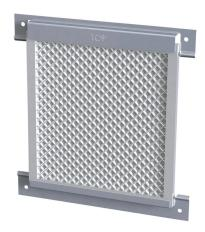
Saginaw filter, replacement, 4.09 x 3.25in, aluminum mesh, aluminum frame, washable. For use with SCE-AVK34 and SCE-AVK34SS.
