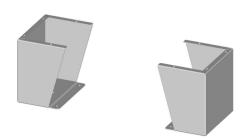
Saginaw floor stand kit, 24in height, 316L stainless steel, #4 brush finish. For use with 12in deep enclosures. Includes (2) floor stands and mounting hardware.
