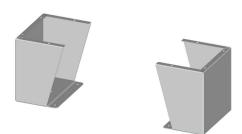
Saginaw floor stand kit, 15in height, 316L stainless steel, #4 brush finish. For use with 24in deep enclosures. Includes (2) floor stands and mounting hardware.
