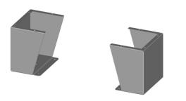
Saginaw floor stand kit, 15in height, carbon steel, ANSI 61 gray, powder coat finish. For use with 12in deep enclosures. Includes (2) floor stands and mounting hardware.
