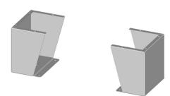
Saginaw floor stand kit, 12in height, carbon steel, RAL 7035 light gray, powder coat finish. For use with 16in deep enclosures. Includes (2) floor stands and mounting hardware.
