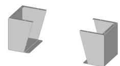
Saginaw floor stand kit, 12in height, 304 stainless steel, #4 brush finish. For use with 10in deep enclosures. Includes (2) floor stands and mounting hardware.
