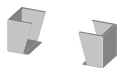
Saginaw floor stand kit, 6in height, carbon steel, RAL 7035 light gray, powder coat finish. For use with 24in deep enclosures. Includes (2) floor stands and mounting hardware.
