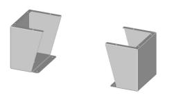
Saginaw floor stand kit, 6in height, carbon steel, RAL 7035 light gray, powder coat finish. For use with 10in deep enclosures. Includes (2) floor stands and mounting hardware.
