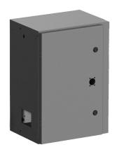
Saginaw external rotary disconnect enclosure,  $48.00 \times 17.00 \times 18.00$  in (HxWxD), carbon steel, ANSI 61 gray, NEMA 3R/12/13. Galvanized subpanel, cable-operated mechanical interlock and mounting hardware included.
