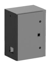
Saginaw add-on rotary disconnect enclosure, NEMA 3R/12/13, door, 24 x 17 x 12in (HxWxD), external mount, carbon steel, ANSI 61 gray, powder coat finish, single-door, 1/4-turn semi-flush, galvanized subpanel included.
