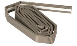
Saginaw EMI/RFI shielded strip gasket, self-adhesive, closed-cell urethane wrapped in nickel-plated copper fabric, 1/4in thick x 1in wide x 7ft long roll. For use with NEMA 4/4X enclosures.
