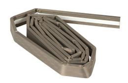
Saginaw EMI/RFI shielded strip gasket, self-adhesive, closed-cell urethane wrapped in nickel-plated copper fabric, 1/4in thick x 1in wide x 7ft long roll. For use with NEMA 4/4X enclosures.
