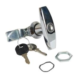
Saginaw enclosure latch, replacement, keylocking, 1/4-turn tee handle, 1-point, die-cast zinc, chrome finish. For use with Enviroline series enclosures. (1) SCE-102804 cam and (2) SCE-K333 keys included.
