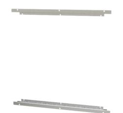
Saginaw horizontal flush-mounting frame flange, 316L stainless steel, #4 brush finish. Package of 2. For use with 30in (W) Enviroline series wall-mount enclosures.
