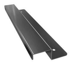
Saginaw enclosure drip shield, 72in length, 304 stainless steel, #4 brush finish. Mounting hardware included.
