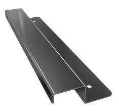
Saginaw enclosure drip shield, 24in length, 316L stainless steel, #4 brush finish. Mounting hardware included.
