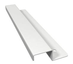
Saginaw enclosure drip shield, 12in length, carbon steel, RAL 7035 light gray, powder coat finish. Mounting hardware included.
