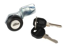
Saginaw enclosure latch, replacement, keylocking, 1/4-turn, 1-point, die-cast zinc, black matte finish. For use with Enviroline series enclosures. (1) SCE-102804 cam and (2) SCE-K333 keys included.
