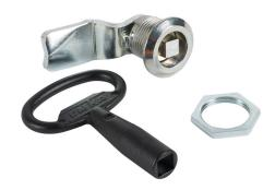
Saginaw enclosure latch, replacement, 8mm square, 1/4-turn, 1-point, die-cast zinc, chrome finish. For use with Enviroline series enclosures. (1) SCE-102804 cam and (1) SCE-101697 key included.
