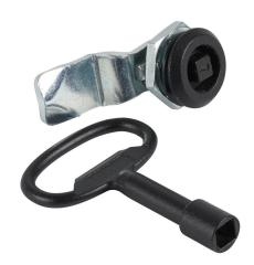
Saginaw enclosure latch, replacement, 8mm square, 1/4-turn, 1-point, die-cast zinc, black matte finish. For use with Enviroline series enclosures. (1) SCE-102804 cam and (1) SCE-101697 key included.
