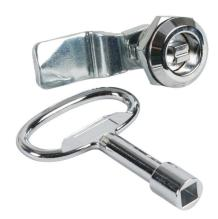
Saginaw enclosure latch, replacement, 7mm square, 1/4-turn, 1-point, die-cast zinc, chrome finish. For use with Enviroline series enclosures. (1) SCE-102804 cam and (1) SCE-101695 key included.
