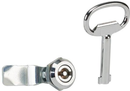
Saginaw enclosure latch, replacement, 5mm double-bit, 1/4-turn, 1-point, vibration-proof, die-cast zinc, chrome finish. For use with Enviroline series enclosures. (1) SCE-102804 cam and (1) SCE-110047 key included.
