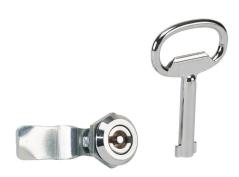
Saginaw enclosure latch, replacement, 5mm double-bit, 1/4-turn, 1-point, vibration-proof, die-cast zinc, chrome finish. For use with Enviroline series enclosures. (1) SCE-102804 cam and (1) SCE-110047 key included.
