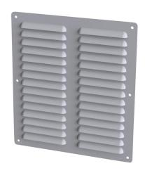
Saginaw louver vent, 10.56 x 9.50in (HxW), carbon steel, ANSI 61 gray, powder coat finish, 9.31 x 8.00in (HxW) cutout, for ventilation of metal enclosure. Mounting hardware included.
