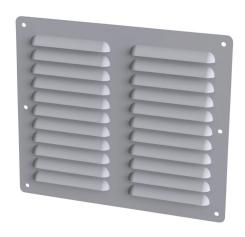
Saginaw louver vent, 8.18 x 9.50in (HxW), carbon steel, ANSI 61 gray, powder coat finish, 6.94 x 8.00in (HxW) cutout, for ventilation of metal enclosure. Mounting hardware included.
