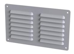
Saginaw louver vent, 5.91 x 9.50in (HxW), carbon steel, ANSI 61 gray, powder coat finish, 4.56 x 8.00in (HxW) cutout, for ventilation of metal enclosure. Mounting hardware included.
