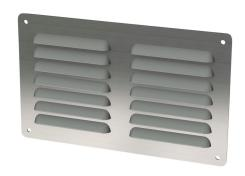
Saginaw louver vent, 5.91 x 9.50in (HxW), 304 stainless steel, #4 brush finish, 4.56 x 8.00in (HxW) cutout, for ventilation of metal enclosure. Mounting hardware included.
