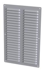
Saginaw louver vent, 15.31 x 9.50in (HxW), carbon steel, ANSI 61 gray, powder coat finish, 14.06 x 8.00in (HxW) cutout, for ventilation of metal enclosure. Mounting hardware included.
