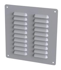
Saginaw louver vent, 7.88 x 7.50in (HxW), carbon steel, ANSI 61 gray, powder coat finish, 6.62 x 6.00in (HxW) cutout, for ventilation of metal enclosure. Mounting hardware included.
