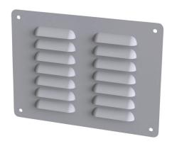
Saginaw louver vent, 5.63 x 7.50in (HxW), carbon steel, ANSI 61 gray, powder coat finish, 4.38 x 6.00in (HxW) cutout, for ventilation of metal enclosure. Mounting hardware included.
