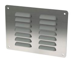
Saginaw louver vent,  $5.63 \times 7.50$ in (HxW),  $304 \times 10^{-2}$  stainless steel, #4 brush finish,  $4.38 \times 6.00$ in (HxW) cutout, for ventilation of metal enclosure. Mounting hardware included.
