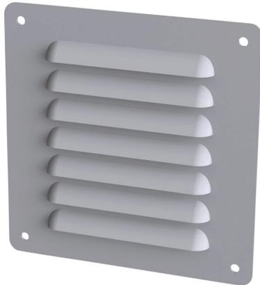
Saginaw louver vent, 5.63 x 5.50in (HxW), carbon steel, ANSI 61 gray, powder coat finish, 4.38 x 4.00in (HxW) cutout, for ventilation of metal enclosure. Mounting hardware included.
