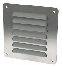
Saginaw louver vent, 5.63 x 5.50in (HxW), 304 stainless steel, #4 brush finish, 4.38 x 4.00in (HxW) cutout, for ventilation of metal enclosure. Mounting hardware included.
