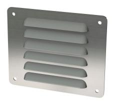
Saginaw louver vent, 4.50 x 5.50in (HxW), 304 stainless steel, #4 brush finish, 3.25 x 4.00in (HxW) cutout, for ventilation of metal enclosure. Mounting hardware included.
