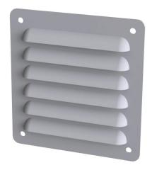
Saginaw louver vent,  $4.75 \times 4.50$ in (HxW), carbon steel, ANSI 61 gray, powder coat finish,  $3.50 \times 3.00$ in (HxW) cutout, for ventilation of metal enclosure. Mounting hardware included.
