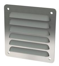
Saginaw louver vent,  $4.75 \times 4.50$ in (HxW), 304 stainless steel, #4 brush finish,  $3.50 \times 3.00$ in (HxW) cutout, for ventilation of metal enclosure. Mounting hardware included.
