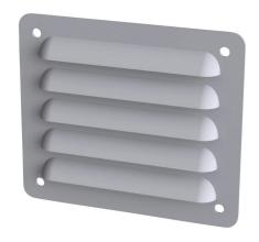
Saginaw louver vent, 3.88 x 4.50in (HxW), carbon steel, ANSI 61 gray, powder coat finish, 2.62 x 3.00in (HxW) cutout, for ventilation of metal enclosure. Mounting hardware included.
