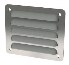
Saginaw louver vent,  $3.88 \times 4.50$ in (HxW), 304 stainless steel, #4 brush finish,  $2.62 \times 3.00$ in (HxW) cutout, for ventilation of metal enclosure. Mounting hardware included.
