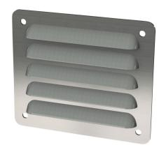
Saginaw louver vent, 3.88 x 4.50in (HxW), 304 stainless steel, #4 brush finish, 2.62 x 3.00in (HxW) cutout, for ventilation of metal enclosure. Mounting hardware included.
